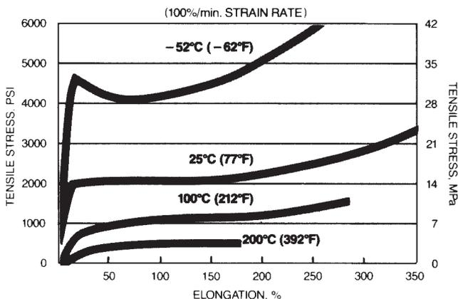
**Figure 2: Tensile Properties of DuPont FEP Film vs. Temperature**
