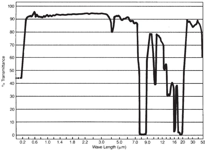
Figure 15: Transmittance at Normal Incidence of Solar Radiation through DuPont FEP Films for Various Thicknesses
